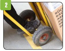
Block the sack trolley with one foot to prevent it from moving backwards.
